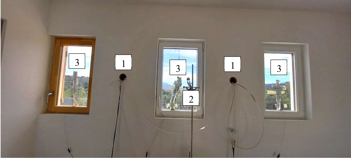
Figure 2: Photograph of the instruments taken from inside the building. 1: pair of total and radiant heat flux gauges. 2: radiant heat flux gauge. 3: K-type surface thermocouple.
